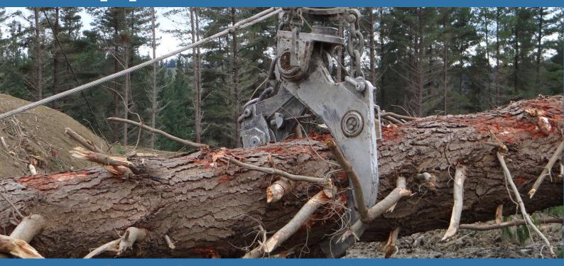
The Brightwater Swing Yarder Grapple is engineered specifically for New Zealand Logging conditions. It features a 2.8 metre jaw opening, heavy Bisolly construction and induction hardened pins. The Grapple's Jaw is also shaped to provide excellent log bunching.
